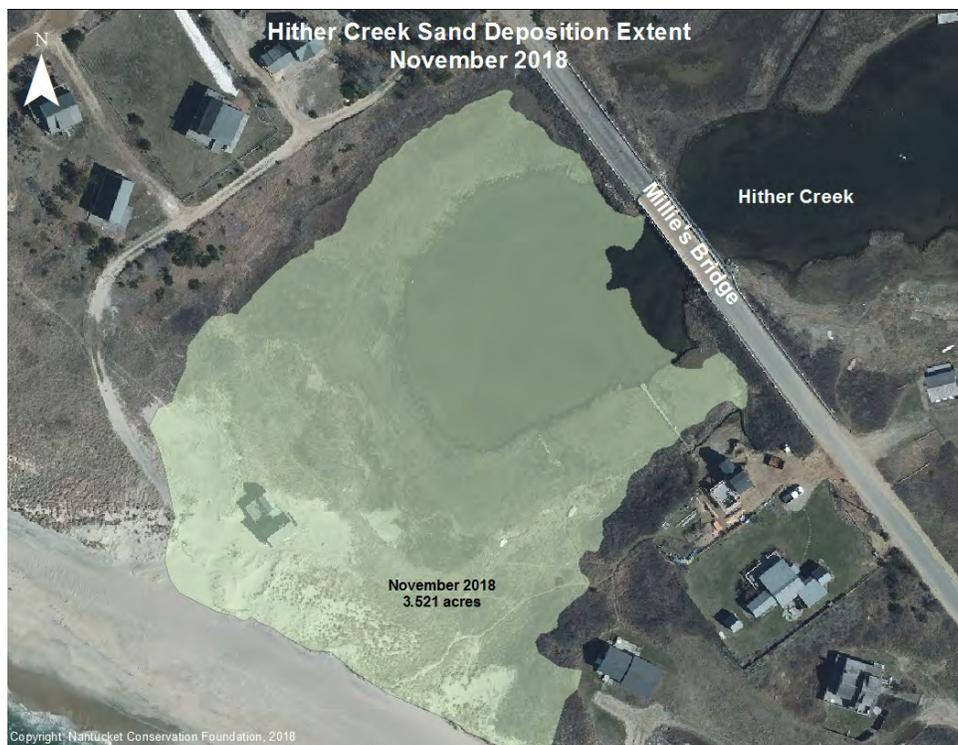
**Figure 3:** Sand extent at Hither Creek and Millie's Pond after 1 year. Daily tides and additional storm wash-overs caused the initial sand deposits to shift and migrate over a larger area.
